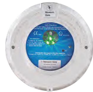
Pulsing LEDs confirm positive ground connection.
