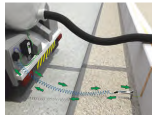
Continuous Ground Loop Monitoring check
