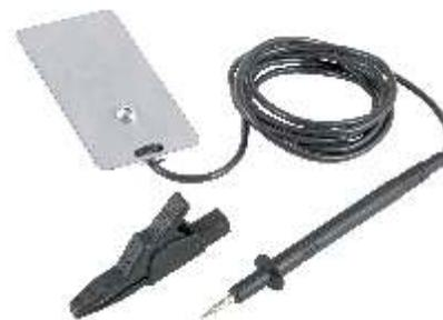
The extension assembly consists of an alligator clip, a test probe and stainless steel plate. It is ideal for testing equipment that does not have a large enough surface to connect to with the OhmGuard clamp. The person performing the test simply connects the OhmGuard's clamp contacts to the plate and then connects the probe or alligator clip to the equipment being tested.
