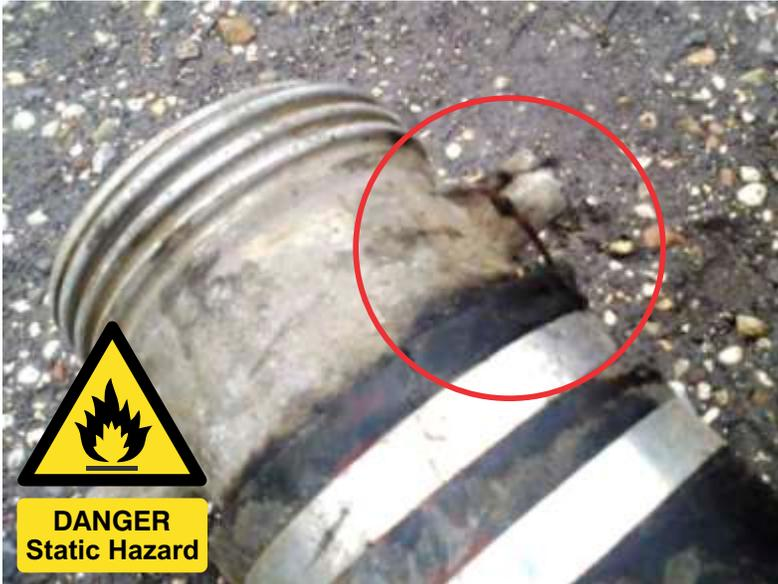
The metal helical wires that reinforce hoses against discharge and suction pressures are commonly used to provide an electrical bond between the end fittings or couplings of hoses. It is important to ensure that wires, like the one illustrated, do not break as this will result in the presence of isolated conductors that have the potential to discharge electrostatic sparks repeatedly during material transfer operations.
