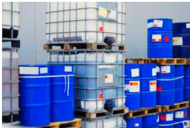
If electrostatic charge is permitted to accumulate the voltage of the IBC will rise very rapidly and result in this energy being discharged in the form of an electrostatic spark onto a grounded object like an operator. If the spark energy is sufficiently high it will ignite the surrounding vapors with little effort. A discharge at 20,000 volts would be capable of releasing up to 60 mJ of energy via the static spark.
