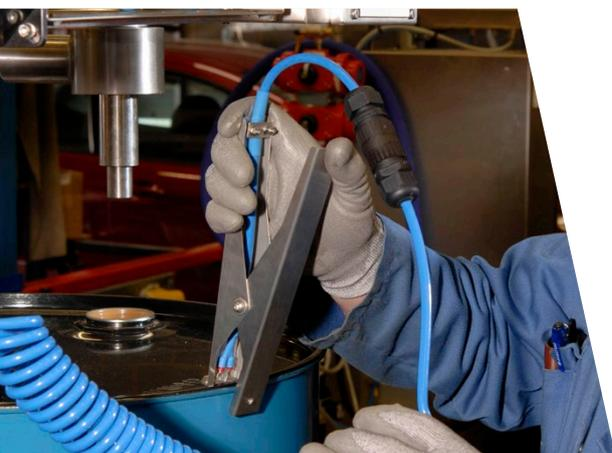
To remove static electricity from the EX/HAZLOC atmosphere grounding clamps should be capable of achieving connections to equipment with resistance values that do not exceed 10 Ohms in the overall system.
