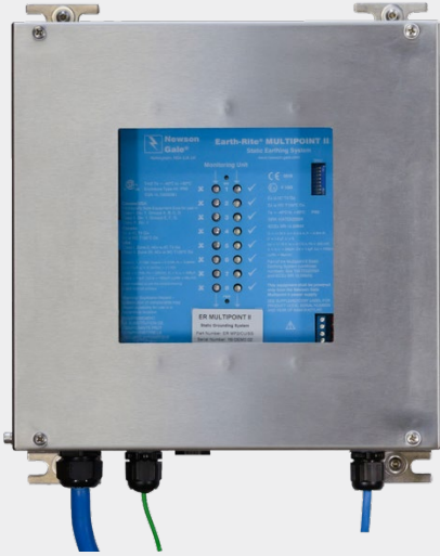
The Earth-Rite MULTIPOINT II's monitoring unit contains 8 pairs of LED ground status indicators (red and green).
