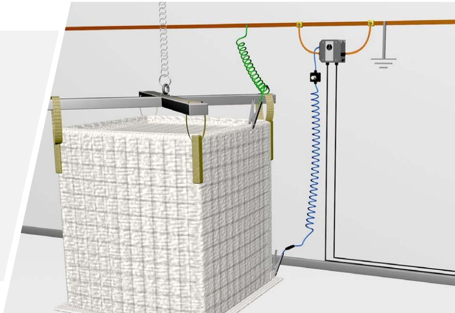
Typical Earth-Rite II FIBC installation consisting of two grounding clamps that establish a continuous ground monitoring loop with the site's locally verified true earth ground source.
