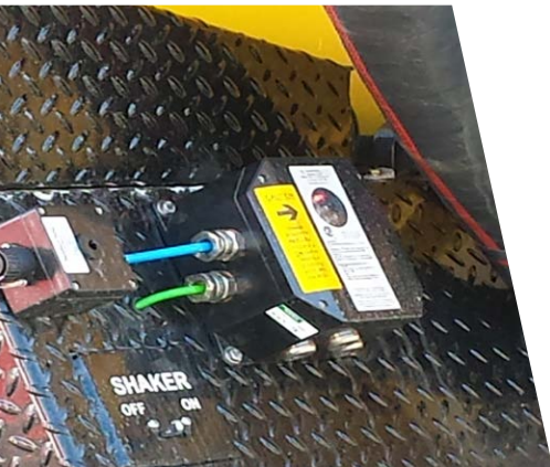
The Earth-Rite II MGV static grounding system can be mounted on vacuum trucks and tank trucks.
