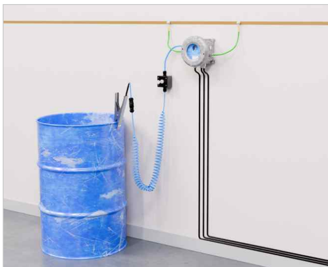
Temporary “ground loop” connection made to metal drum prior to a filling or blending operation. The copper tape is connected to the plant’s verified earth.
